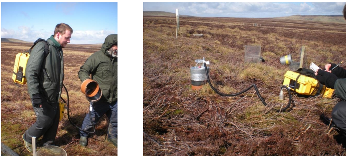
Figure 3 Hands-on measurements: field deployment of gas flux chambers for measuring greenhouse gas emissions (GHGs) using latest analyser technology (Los Gatos) for measuring net methane (CH 4 ) emissions in the field.
