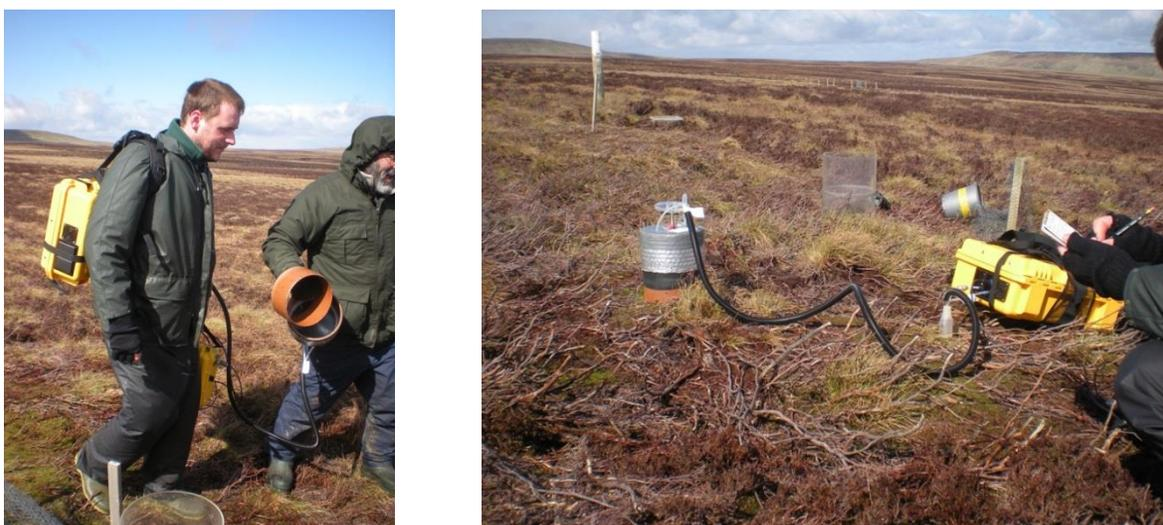
**Figure 3 Hands-on measurements:** field deployment of gas flux chambers for measuring greenhouse gas emissions (GHGs) using latest analyser technology (Los Gatos) for measuring net methane (CH<sub>4</sub>) emissions in the field.
